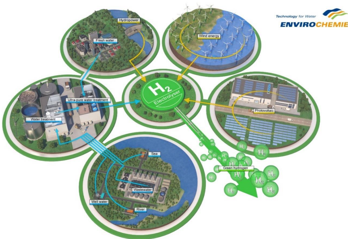
Figure 1: Integration of industrial wastewater and other feedstock water sources into a holistic approach for hydrogen production
