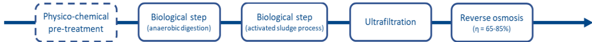
Figure 5: Flow diagram of wastewater recycling treating wastewater with a high organic load.
