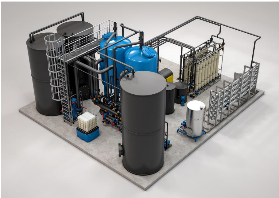
Figure 4: 3D model of the installed plant producing 188,000 \text{m}^3 per year of water in drinking water quality using cow water as a water source.
