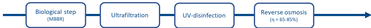
Figure 3: Flow diagram of the treatment strategy for treating organically low-polluted streams to drinking water quality.
